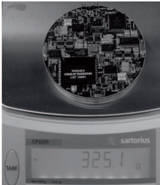
Figure 19. Photograph of the completed COSA propulsion system with wireless telemetry, inertial measurement unit and thrust control electronics on a weight scale.
