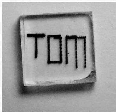
Figure 10. (a) Absorption spectra of a sodium chloride sample before and after darkening by 400-nm, femtosecond laser irradiation. (b) A Professor Made coloration of NaCl (the dots are single pulses) by scanning the laser beam by hand.
